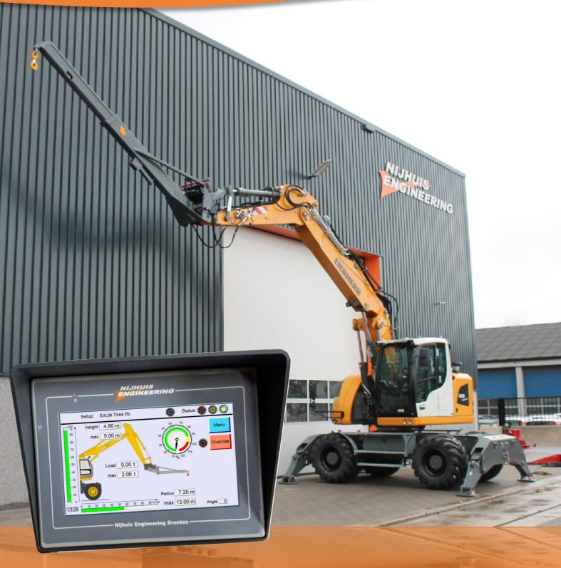
Rated Capacity Limiter for hoisting excavators conform EN 13000
